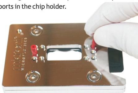
Figure 2.3. Screw the alignment nuts gently into the chip holder
