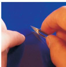
Figure 2.5. Cutting the capillary
