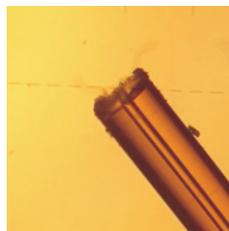
Figure 2.6. Capillary that has been cut
