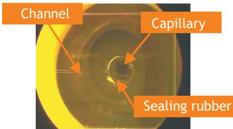
Figure 2.9. Capillary correctly positioned above the channel
