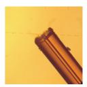
Figure 2.6. Capillary that has been cut
