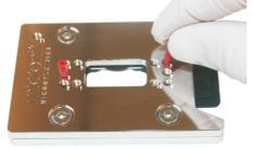
Figure 2.3. Screw the alignment nuts  $\underline{gently}$  into the chip holder
