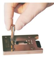
Figure 5.1. Extender tool, for 1/4 or 1/3 round additional tightening
