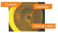
Figure 2.9. Capillary correctly positioned above the channel
