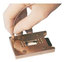
Figure 2.12. Threaded hole for the assembly of 'Flat-Bottom' fittings
