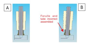
Figure 5.2. Assembly of tubing and ferrule
